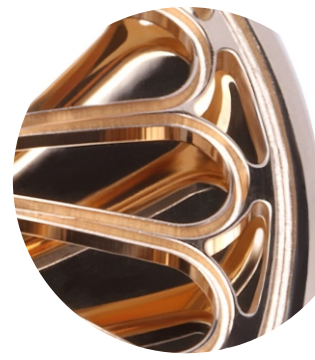
Milling of finest channels in a jewelry pendant
